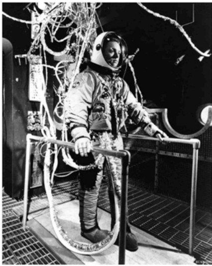
NASA, "Portable Life Support System, Successful Apollo EMU Chamber Testing (Courtesy United Technologies Aerospace Systems)", USA, 1965
